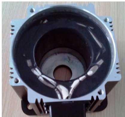
After Sealant Filling
